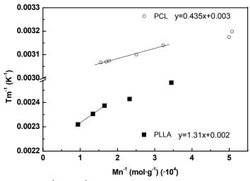
**Figure 13.**  $T_m^{-1}$  vs Mn<sup>-1</sup> Flory relationship for PLLA and PCL. The intercept of the y-axis is  $\frac{1}{T_m^{\infty}}$ .
