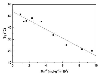
**Figure 12.** Tg versus Mn<sup>-1</sup> Flory-Fox relationship for PLLA polymers. The intercept of the y-axis is  $T_g^{\infty}$ .
